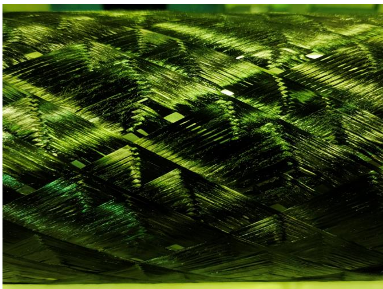
Figure 4. Gaps (space) between the bundles
